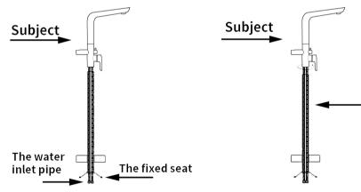
3. Screw and hand tighten the water inlet pipe to the water inelets of the subject (DO NOT USE SPANNER TO TIGHTEN AS IT CAN DAMAGF THE O-RING) Make sure the water inlet pipe were screwed into the correct inlets for hot water and cold water.
