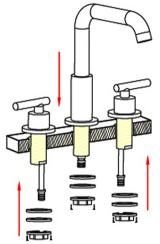
2. Place the faucet body and handles into sink holes. screw the plastic washer, metal washer and locking nut to the thread pipe of the faucet as photo 2
