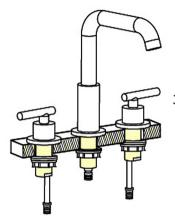
3. Adjust the position of the faucet and the handles then hand tighten the locking nut and then use a screwdriver to tighten the screws on the locking nuts to secure the faucet
