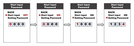
You need to input the right password before start with 30 seconds, display will power off automatically if the password was wrong.
