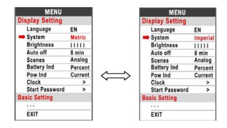
**Brightness**: Press Up / Down button to change the brightness of the backlight, I is darkness, IIIII is brightness.
