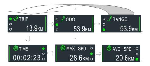
\*\*If there is no operation for 5 seconds, display will return Speed (Real-Time) display automatically.
