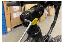
After tightening the 2 side bolts, firmly tighten the top bolt. After all 3 bolts have been securely fastened, make sure there is no play in the headset by tighten the 4 pinch screws with 4mm Allen key. Loctite is recommend on the screw Align the brake controls so they are facing slightly downward. Fine tune the position to align with your arm when seated, stem rise angle can be adjusted by loosen the big side screw with 6mm Allen key
