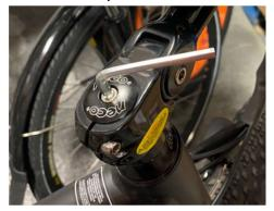
Once the handlebars are aligned and the top bolts is slightly secured, firmly tighten the 2 side bolts with **5mm Allen key** on the stem.
