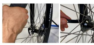
6) Install the headlight to the front fork with the given long bolt and nut, tighten with the **5mm Allen key** and **10mm wrench**
