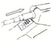
• Plug the three prong side into the battery socket. Keep in mind the orientation of the plug and socket so they are aligned properly.
