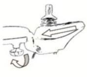
•Insert the controller joystick into the armrest tube and tighten the knob to fix it in position
