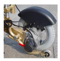
Before the user is seated in the chair, put down the red brakes which are near the rear wheels.
