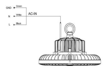
Turn off the power connect black wire to L, white wire to N, and green wire to G (details as below), then turn on the power.
