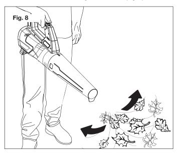
Slowly advance the unit, keeping the accumulated pile of debris in front of you.
