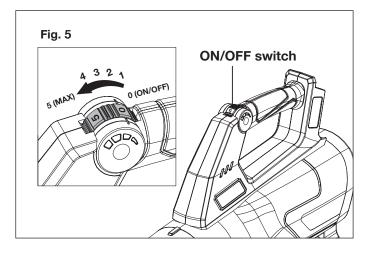
**3.** This unit is equipped with 5 variable speed settings. Position "5" is the maximum setting blow up to 100 mph (Fig. 6).
