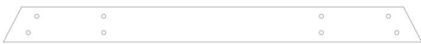
M82 | PLANCHE DE SOL DE BARRE DE SINGE - W4L13850 (1) 5/8"x3 3/8"x39 5/8" (16x86x1006)
