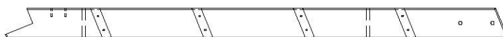
E15 | MONTANT GAUCHE - W4L13322 (x1) | 1 3/8 po x 3 3/8 po x 56 3/4 po (36 x 86 x 1441)
