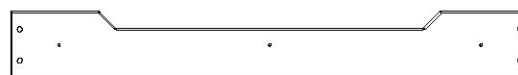
K10 | RAIL MURAL - W4L13174 (x1) | 5/8 po x 5 1/4 po x 40 1/2 po (16 x 134 x 1030)
