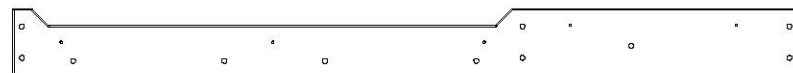
G2 | RAIL MURAL - W4L13171 (x1) | 1 po x 5 1/4 po x 61 3/8 po (24 x 134 x 1560)
