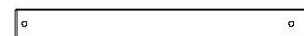
J12 | RAIL MURAL - W4L13188 (x2) | 1 po x 2 3/8 po x 23 1/4 po (24 x 60 x 590)
