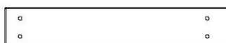
L3 | RAIL MURAL - W4L13189 (x1) | 5/8 po x 4 3/8 po x 24 7/8 po (16 x 112 x 631)
