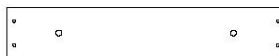
H82 | PLANCHE DE FIXATION - W4L14553 (x1) | 1 po x 3 3/8 po x 18 1/4 po (24x86x462)
