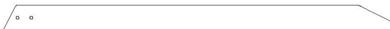
H2 | CALE DE LA BARRE DE SUSPENSION - W4L14544 (x2) | 1 po x 3 3/8 po x 51 1/2 po (24x86x1308mm)
