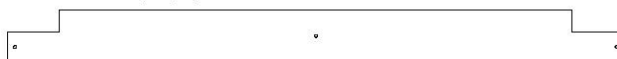
M5 | PLANCHE DE PLANCHER - W4L14575 (x1) | 5/8 po x 3 3/8 po x 40 3/8 po (16x86x1024)
