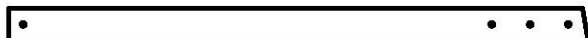
E71 | RAIL DE BARRE DE SUSPENSION - W4L06929 (x1) | 1 3/8 po x 3 3/8 po x 60 5/8 po (36x86x1539)
