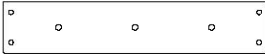
M77 | CALE DU TOBOGGAN - W4L08748 (x1) | 5/8 po x 3 3/8 po x 17 1/4 po (16x86x438)
