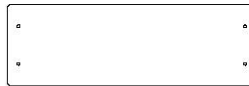
K6 | PLANCHE DE MUR - W4L14562 (x1) | 5/8 po x 5 1/4 po x 16 1/4 po (16x134x412)
