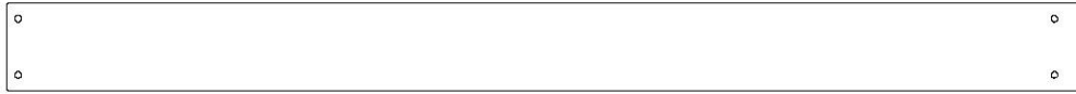
K1 | PLANCHE DE SOL - W4L14557 (x2) | 5/8 po x 5 1/4 po x 64 3/4 po (16x134x1644)
