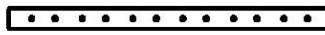
O1 | TASSEAU DE PORTE - W4L14609 (x3) | 5/8 po x 1 3/8 po x 21 po (16x34x534)
