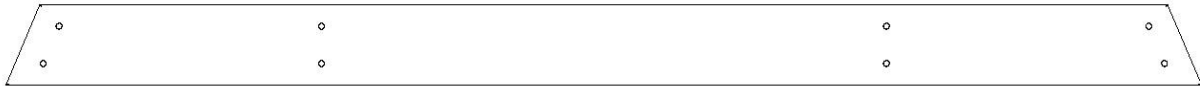
K4 | PLANCHE DE SOL - W4L14560 (x1) | 5/8 po x 5 1/4 po x 78 1/4 po (16x134x1986)
