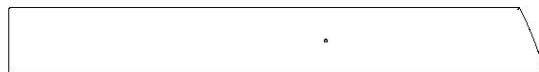
L8 | PLANCHE DE PORTE - W4L14570 (x1) | 5/8 po x 4 3/8 po x 35 po (16x110x890)
