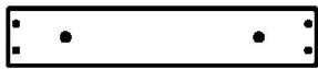
H82 | PLANCHE DE FIXATION - W4L14553 (x1) | 1 po x 3 3/8 po x 18 1/4 po (24x86x462)
