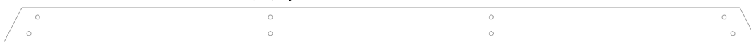
H3 | PLANCHE DE SOL DE BARRE DE SINGE - W4L14545 (x1) | 1"x3 3/8"x70 3/8" (24x86x1786)
