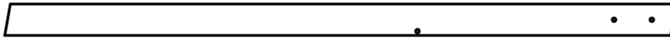
E6 | MONTANT DE LA BARRE DE SINGE - W4L14536 (x1) | 1 3/8"x3 3/8"x71 3/8" (36x86x1812)
