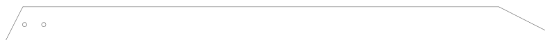
H2 | CALE DE BARRE DE SINGE - W4L14544 (x2) | 1"x3 3/8"x51 1/2" (24x86x1308 mm)
