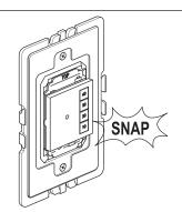
NOTE - If you need to remove switch after snapping into frame, first remove frame from wall box to access the four locking tabs on the back of the switch. Insert a flat screwdriver to depress tabs as you apply pressure to push sensor out.
