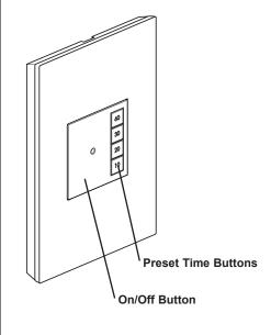
The adorne SensaSwitch - Manual ON/Timed OFF turns OFF the connected light when the selected time expires.
