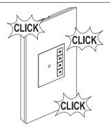
NOTE - To remove wall plate, insert a small, flat screwdriver in notches on wall plate and twist gently to pry from frame.
