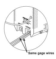
NOTE:When two wires connect to the same terminal on the sensor, both wires must be the same gage (12AWG or 14AWG.) If they are not the same gage, you will not have a secure connection
