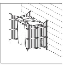
\* Screens are designed to be installed at a right angle for optimal stability. If installing in a straight line or independently from each other, it is recommended to secure the posts into the ground with a bit of gravel or quick drying cement to ensure your screens are not easily knocked over.
