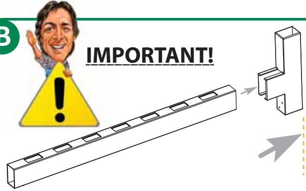
B - Insert top rail ALL THE WAY until it BOTTOMS OUT inside bracket
