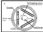
1. To reduce the risk of electric shock, ensure electricity has been turned off. Install the chassis on the ceiling with a self-tapping screw; if the lamp is not installed firmly, it will cause the lamp to fall off and entail a loss.
