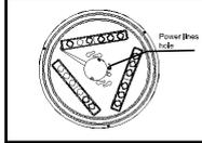
2. Choose the right wire (0.75-1.5mm<sup>2</sup>) and connect the wire properly; if not, it will cause easily the fire and other accidents.
