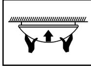
3. Install the diffuser by rotating it until securely fastened. Ensure the diffuser is screwed and secured properly. An improperly installed diffuser may fall.
