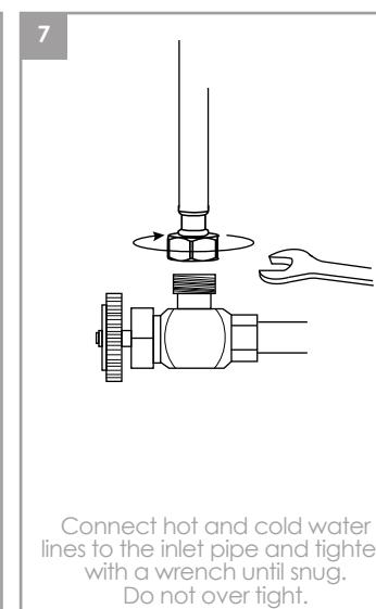
Connect hot and cold water lines to the inlet pipe and tighten with a wrench until snug. Do not over tight.
