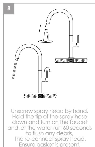
Unscrew spray head by hand. Hold the tip of the spray hose down and turn on the faucet and let the water run 60 seconds to flush any debris, the re-connect spray head. Ensure gasket is present.
