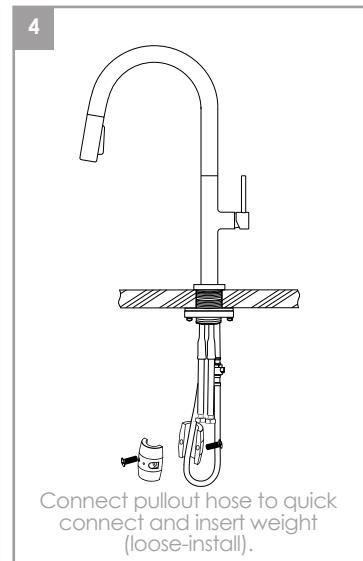
Connect pullout hose to quick connect and insert weight (loose-install).
