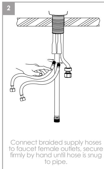
Connect braided supply hoses to faucet female outlets, secure firmly by hand until hose is snug to pipe.
