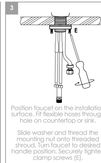
Position faucet on the installation surface. Fit flexible hoses through hole on countertop or sink.
