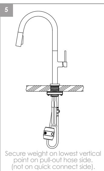
Secure weight on lowest vertical point on pull-out hose side. (not on quick connect side).
