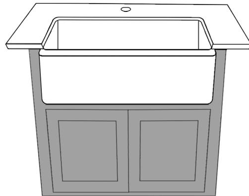
Finish installation of rest of the components the cabinet face and doors to complete the cabinet front, and finish the rest of your plumbing and counter installation. Once your counters are in place, caulk the edges of your sink to prevent water penetration to the inside of the cabinet.
