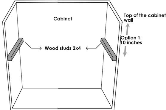
Cut your 2x4 to size and install on the left, right wall of the cabinets, ensure they are leveled and allow space for doors.
