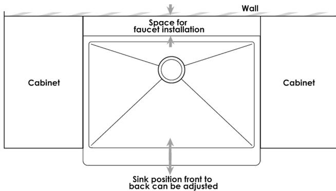
Rest your sink on the supports and check if it is level and flush. For the position front to back, Stylish sinks have a side faces that are full cover, so sink position can be adjusted to leave good space for faucet installation.
