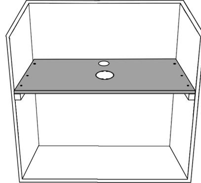
If the width of the cabinet is too large you need to add plywood shelf on top of the 2x4, so the position of the 2x4 should be lower and offset by the thickness of the shelf, in this case is recommended to add a 2x4 at the rear of the cabinet, also shelf will need to have cut-outs to clear the plumbing hoses and drain connections.
