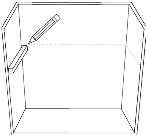
Apron sinks are heavy, install strong support, it is recommended to use 2x4 lumber and add a plywood shelf if the cabinet width is much larger than the sink length.
