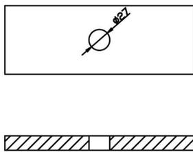
Recommend hole size 25mm to 29mm hole diameter.
