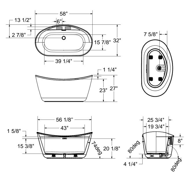
(﴿ Recommended faucet area 2 sections of 6" (L) x 2 7/8" (W). Depth recommended for straight pipes 8".
