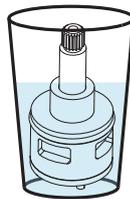
If a cartridge does not respond well, you will need to clean it in a solution of half vinegar and half hot water, ideally overnight, brush and then rinse it under clean water. Apply plumbing grease to the O-rings, replace the cartridge.
