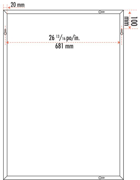
Measure, mark and drill pilot holes where the brackets are to be installed.
