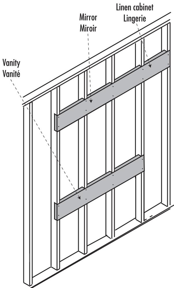
To safely install your vanity, mirror or linen cabinet, strengthen your wall with a 2"x 6". The recommended height for a vanity with bathroom sinks is +/- 34 in. (864 mm). Measure, mark and drill pilot holes where the brackets are to be installed. Consult an expert for the proper screws/bolts to use when attaching to various wall constructions. Screws provided do not attach to all wall construction type.
