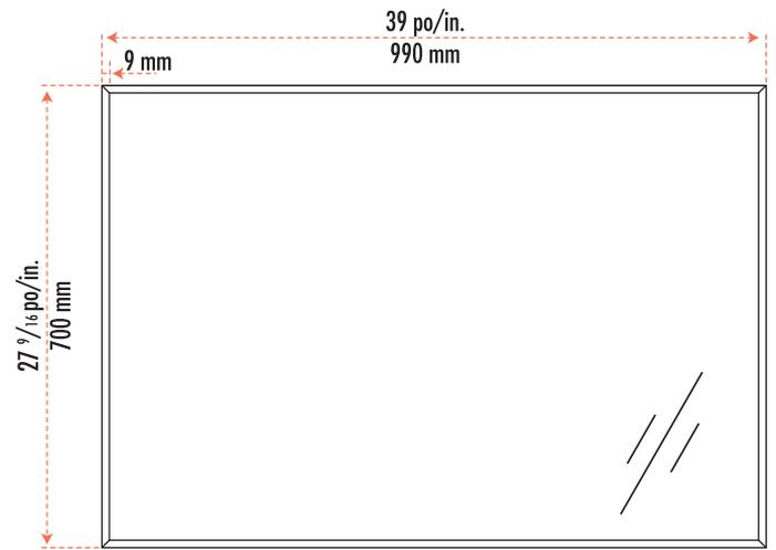
It is recommended to leave a minimum of 10-inch space between the mirror and the sink, and 3 inches between the mirror and the faucet to allow enough space for the handle of the faucet.
