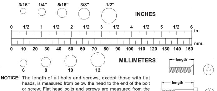
top of the head to the end of the bolt or screw.
