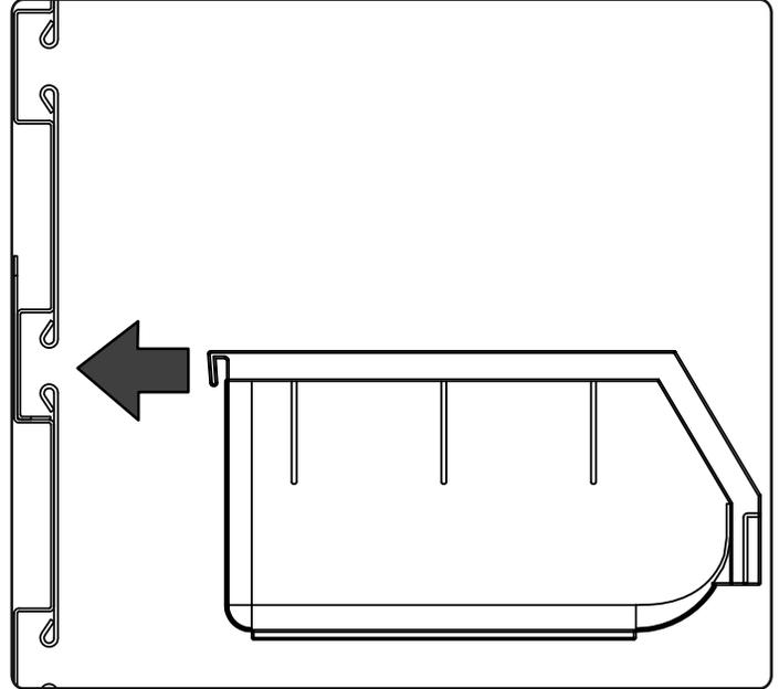
**2** Seat the parts bin by inserting and firmly pressing the top lip onto the Slatwall channel.
