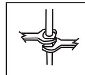
Tighten connection with two wrench to prevent damage to tube body. Be careful not to bend the stem as this will void the product warranty.
