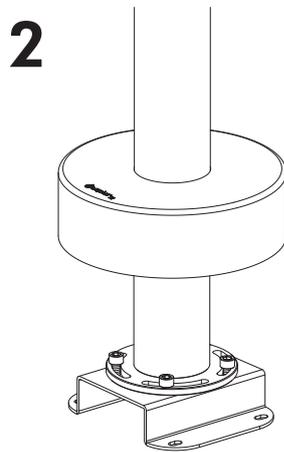
Install the screws by hand and do not overtighten
