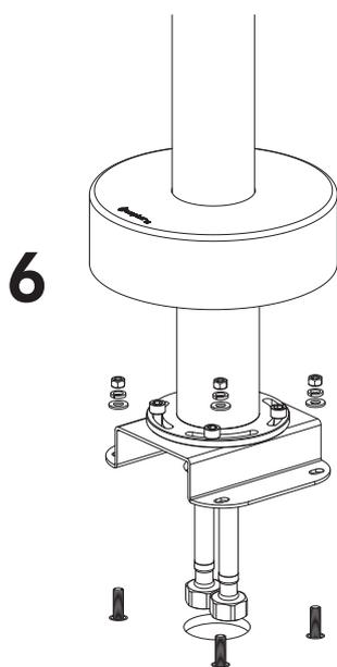
Screw or anchoring the base flange firmly on the floor
