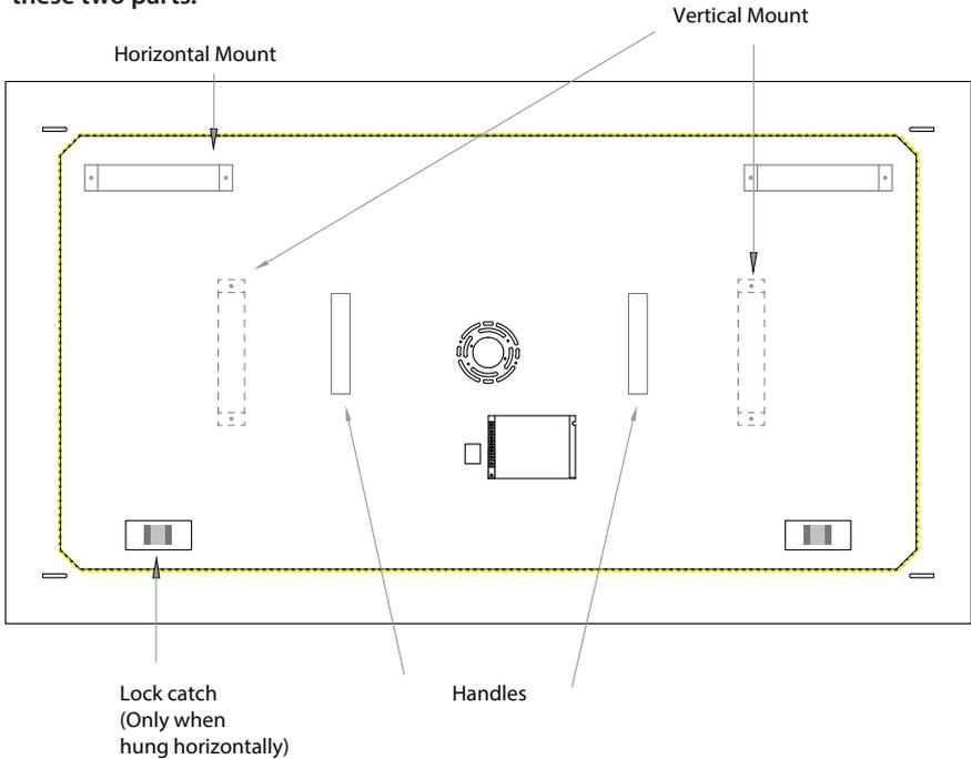
2. Remove the two horizontal mounts on the back of the frame. Line up the holes on the bracket with the holes placed for the vertical mount and screw the bracket in. Remove the two catch locks located at the bottom of the metal frame by removing its screw.
