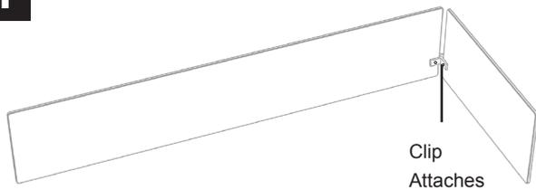
Connect two pieces of glass together with a provided clip. Lightly tighten screws.
