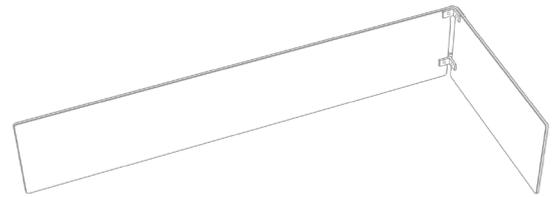
Connect two pieces of glass together with provided clip. Lightly tighten screws.
