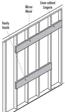
To safely install your linen cabinet, strengthen your wall with a 2''x 6''. Measure, mark and drill pilot holes where the brackets are to be installed. Consult an expert for the proper screws/bolts to use when attaching to various wall constructions. Screws provided do not attach to all wall construction type.
