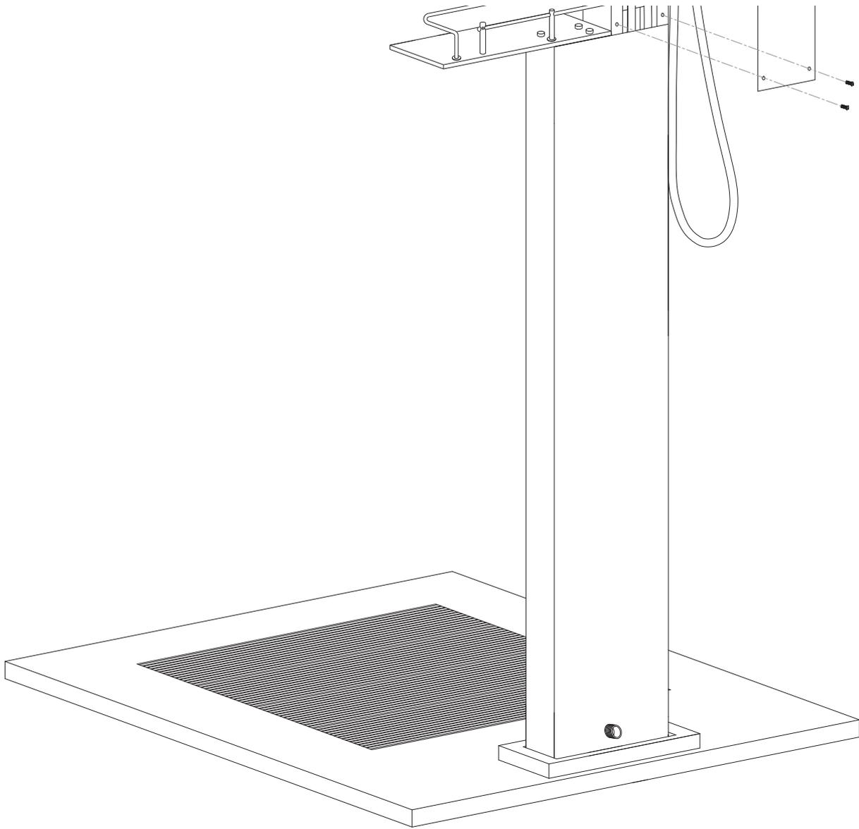
Before you connect the shower panel turn on the water and let it run for at least one minute to clean the pipes and eliminate any dirt that may be stuck there.
