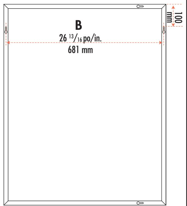
Measure, mark and drill pilot holes where the brackets are to be installed.
