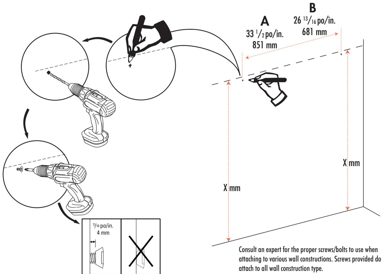
Consult an expert for the proper screws/bolts to use when attaching to various wall constructions. Screws provided do not attach to all wall construction type.
