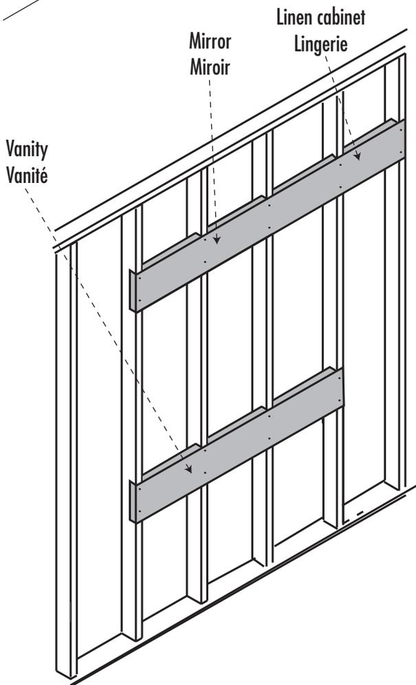
To safely install your vanity, mirror or linen cabinet, strengthen your wall with a 2"x 6". The recommended height for a vanity with bathroom sinks is +/- 43 in. (107 cm). Measure, mark and drill pilot holes where the brackets are to be installed. Consult an expert for the proper screws/bolts to use when attaching to various wall constructions. Screws provided do not attach to all wall construction type.
