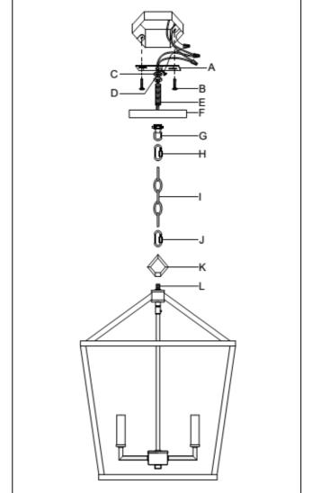
Line art shown may not exactly match the fixture enclosed. However, the installations do apply to this fixture. ITEM NO:3234AS 3234RBZ 3234VG 3234-MB 3234-SN
