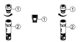
This faucet ships with a 1.8 GPM flow restrictor installed. An optional 2.2 GPM flow restrictor is also included in the box.
