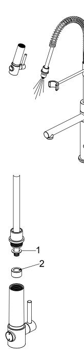
Pull the hose assembly out of the spout and remove the spray head by unscrewing it from the hose in a counterclockwise direction. Be sure to hold the end of the hose down into the sink and turn the faucet on to the warm position where it mixes hot and cold water.
