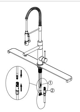
Push the quick connector (2) firmly upward and attach it to the receiving block (1). Pull down moderately to ensure the connection has been made.
