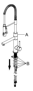
Shut off the water supply. Remove the old faucet. Clean the mounting surface. Remove mounting hardware (B) from faucet body (A).
