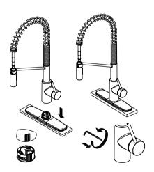
Align arrow on faucet body (B) with arrow on base (J). Attach faucet body (B) to base (J). Secure faucet body (B) by tightening the set screw with 2.5mm hex wrench (i1).
