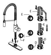
Remove Quick Connect (H) from spray hose (F). Insert spray hose (F) into small hole of base (J). Insert hot & cold waterlines (E) and supply hose (D), one by one, in large hole of base.
