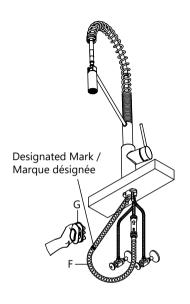
Attach weight (G) on the designated mark on the spray hose (F).
