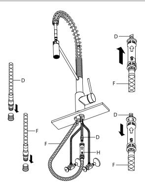
Attach Quick Connect (H) with black end onto spray hose (F) until you hear a click. Attach the other end onto the supply hose (D) until you hear a click.
