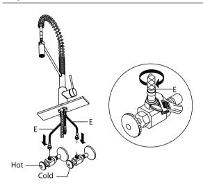
Thread hot & cold waterlines (E) onto angle stops. Tighten with adjustable wrench until snug. Turn on the angle stops and check for leaks.
