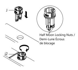
Insert base (J) into sink or countertop with "FR1NT" facing forward. Tighten screws on base (J) with 4mm hex wrench (i2) until base is secure on sink or countertop.
