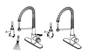
Remove spray head (A). Hold tip of spray hose (F). Turn faucet on for 1 minute to flush any debris. Reconnect spray head (A).
