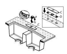
Place the escutcheon (C) and the gasket on the sink. Insert the base (a) into escutcheon (C). Note: "Front" on the base must face the front of the sink. The two mounting plates (b) on the base (a) must be loose and movable during the installation of the base (a). If the sink is uneven, use silicone under the gasket (D).
