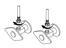
Attach waterlines to angle stops and tighten until snug. Turn on angles stops and check for leaks. (DO NOT TURN FAUCET ON)
