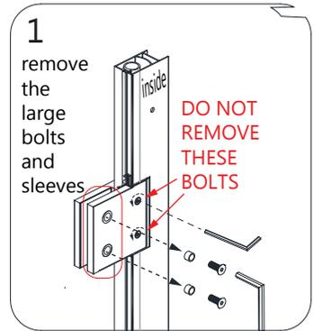
**5. The Hinge Assemblies (#04)** are pre-attached to the **Hinge Profile (#02)**. Remove the **large allen bolts** and protective sleeves from the hinges. **(Fig 5.1)** Loosen the **smaller allen bolts** on the hinges to create enough space to slide the glass into the hinges.
