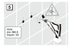
• After holes have been drilled, insert the provided Anchor Screws (Part 15).
