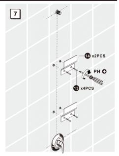
For the Positioning & Mounting Brackets (Part 14), please make sure that they are installed with protruding portion facing upward as shown in the drawing.
