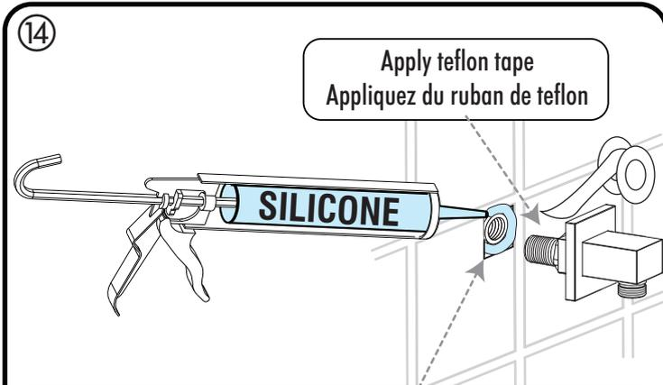
Put silicone to prevent infiltration into the wall
