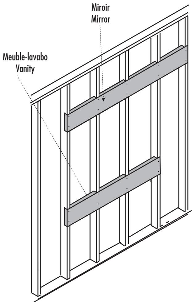
Fix the screws into your wood reinforcement (2 x 6 in. stud or 1/2 in. plywood). Consult an expert for the proper screws/bolts to use when attaching to various wall constructions. Screws provided do not attach to all wall construction type.
