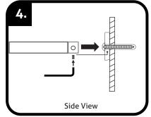
Attach accessory to the mounting plate Use provided hex key to tighten the hex head located on the side of the accessory to secure the product.
