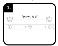
For Towel Bars: Using a level and measuring tape, measure the distance between mounting plates. Mark Screw points with tip of screwdriver or pencil. (For other accessories, skip to step 2)
