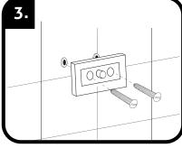
Attach each mounting plate to wall by installing screws into pre-drilled wall anchor holes.
