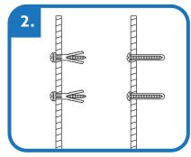
Prepare fastener holes for attaching the mounting plates using options below: A. Attaching to stud in drywall. B. Attaching to drywall.
