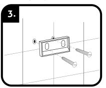
Attach each mounting plate to wall by installing screws into pre-drilled wall anchor holes. (Robe holder accessory must be positioned vertically.)
