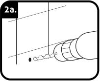
Attaching to stud in drywall: Use drill bit smaller than the screws to pre-drill holes.
