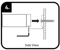
Attach accessory to the mounting plate Use provided hex key to tighten the hex head located on the underside of the accessory to secure the product.
