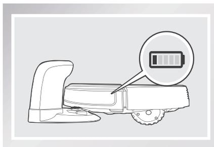
\* Make sure to turn the robot's Bottom Power Switch to the ON position before charging. ("I"=power ON; "O"=power OFF. The robot's default setting is "O".) DEEBOT is powered ON when the AUTO Mode Button glows a continuous BLUE.
