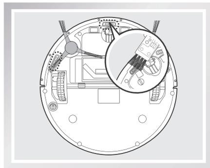
Wipe the robot's Charging Contacts and Charging Docks Pins with the brush of the Multi-Function Cleaning Tool or with a dry cloth to maintain their effectiveness.
