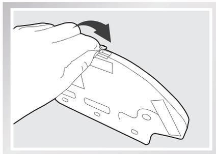
Attach the Advanced Wet/Dry Reservoir to the bottom of the robot. Insert the tabs on the Advanced Wet/Dry Reservoir into the Advanced Wet/Dry Reservoir Slots on the bottom of the robot until you hear a click.
