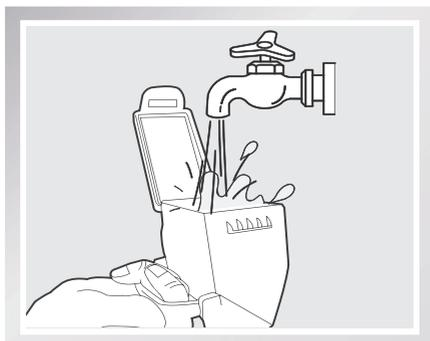
Dry the Dust Bin and filters completely before reinstalling.
