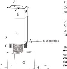
Fix the Upper Chimney (B) to the Ceiling Mount (A) using (4) ST4x6 self tapping screws.
