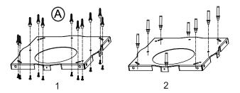
[1] 13 pcs ST4 x 30 Wood Screws + 13 Wall Anchors for Wood Mounting
