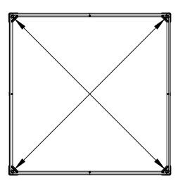
This is important to get square angles in crossbars corners so diagonal measurements (X) should be taken at top of posts in corners and get the same for both. This care refer to get an easy assembly.
