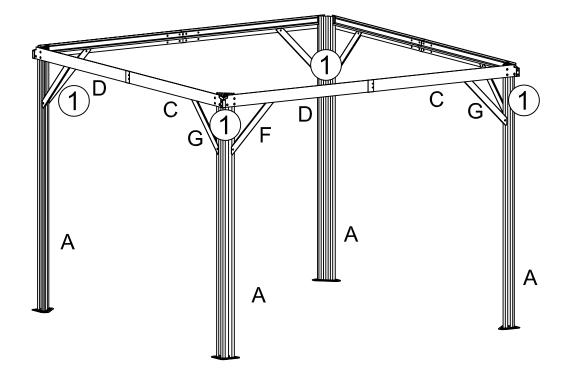
Step 4: Secure left and right braces ( G & F ) to posts ( A ) by using bolts ( AA ) as fig.1 shown. Do not tight bolts yet. Then secure other end of braces ( G & F ) to short and long assembly crossbars ( DC ) by using bolts ( AA ) as fig.1. Prior final tightening, ensure assembly is fully aligned. Then, tight all loose bolts.
