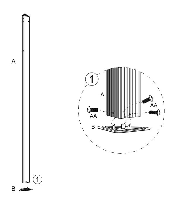
Step 1: Secure base flange (B) to the bottom of post (A) by using bolts (AA). Repeat the step for all rest posts. Bolts can be tight completely.
