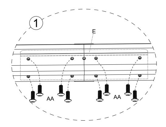
Step 2: 1.Insert the connector (E) into a crossbar (C) and a crossbar (D) as figure shown, and secure with bolts (AA). Bolts can be tight completely.
