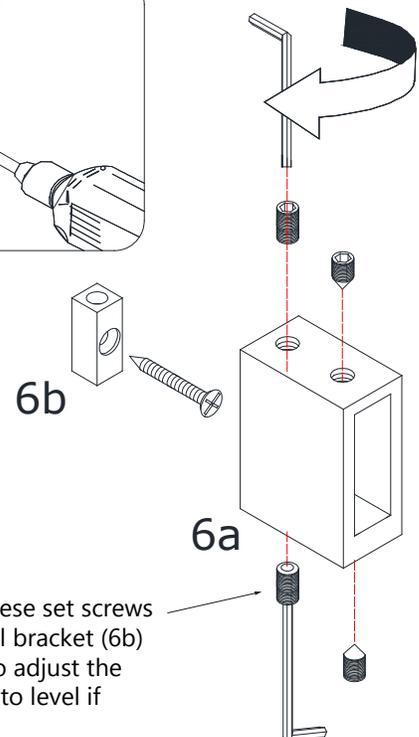
tighten these set screws to the wall bracket (6b) and use to adjust the guide rail to level if necessary
