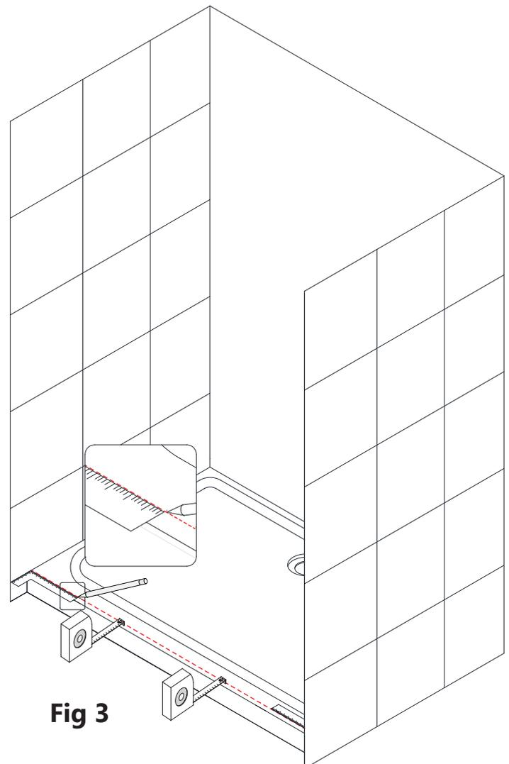
**4.** Align the outside edge of the **U-Channel (#01)** with the inside of the mark on the threshold.
