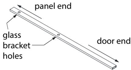
**NOTE:** Use a metal file to remove any burrs from the cut end of the **Guide Rail (#04)**.
