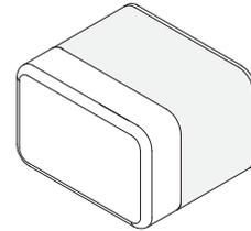
The **Bumper (#26)** is reversible for Left (as shown below from inside the shower) or Right wall installation
