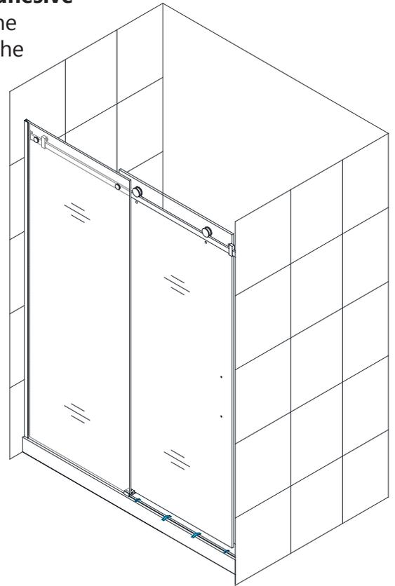
**TIP:** Position the roller guard 1/16" below the guide rail, hold the roller guard bolt with the Allen wrench and tighten the interior post using the small Allen wrench (**Fig 27.2**)
