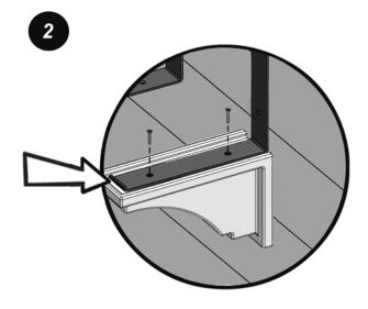
The front lip of the wall mount bracket should sit flush against the inside face of the decorative bracket (indicated by the arrow). The molded brackets are only decorative so there is no need to over tighten the screws.
