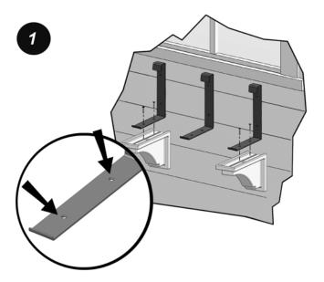
Some window boxes may have wall mount brackets that need pre-drilling. Drill 2 holes about 5 inches apart using a 1/4 inch drill bit. We recommend countersinking the holes so the screw head sits flush with the bracket. Secure each decorative bracket to the bottom of the wall mount brackets using two 1 inch screws.
