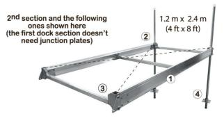
**STEP 2** Insert and bolt-in with 1/4in x 1 1/4in bolts the 2 end extrusions by hand (longer part of leg holder on top). Make certain that angles are straight by taking an 'X' measurement from corner to corner. If both measurements differ more than  $\pm$  4mm (1/8 in), gently push on frame until both measurements are the same, then tighten bolts (BEWARE, aluminum is soft – DO NOT over tighten).
