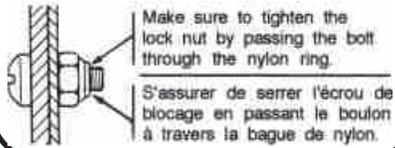
Make sure to tighten the lock nut by passing the bolt through the nylon ring.
