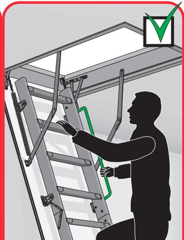
While ascending or descending the ladder, do not hold onto the brackets, springs or other hardware elements of the ladder.
