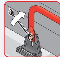
When moving the handrail from the right to the left, use the screws with which it was bolted to the ladder. Additionally, the screws should be well tightened so that the handrail does not break off in the course of later use.
