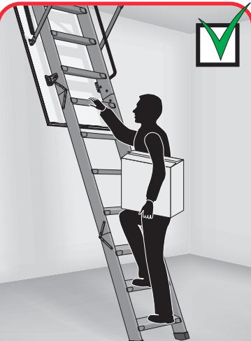
While ascending or descending the ladder, the user should always face the ladder and hold tightly onto the treads or handrail at least with one hand.
