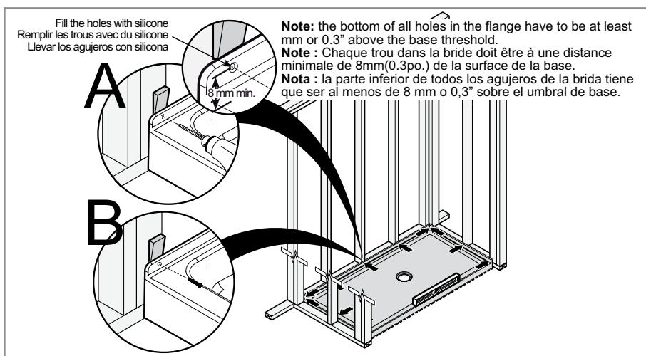
Fasten the base to the studs with # 8 screws by first drilling the mounting flange with a 3/16" bit.
